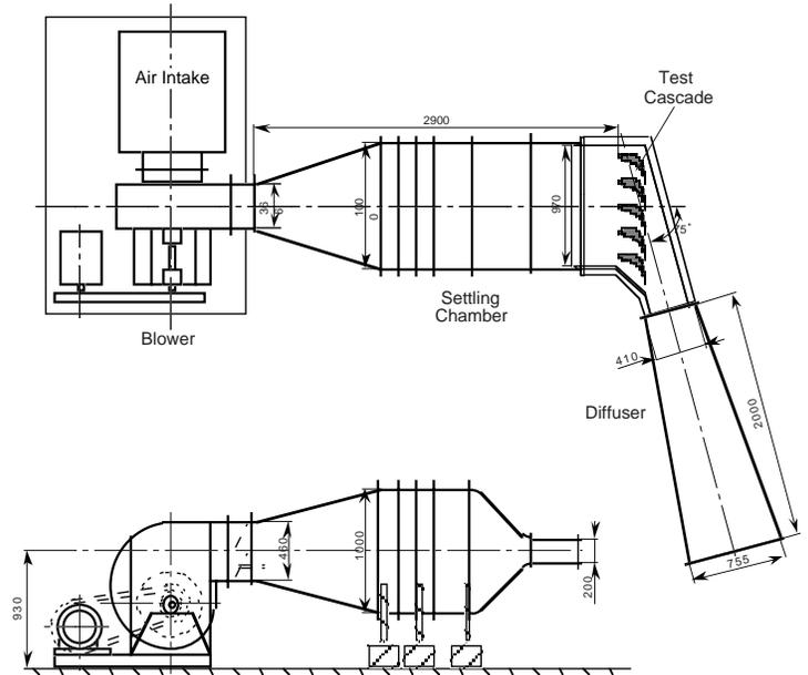
Fig. 2 Schematic layout of the test apparatus
