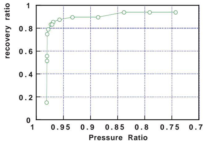
Fig. 7 Water recovery ratio of the suction slit
