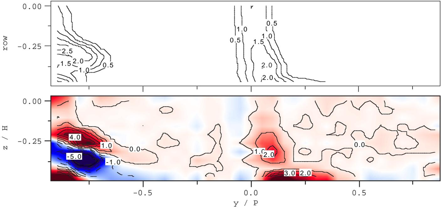
Fig. 10 Measurements of total loss and secondary vorticity (upper) Total loss
