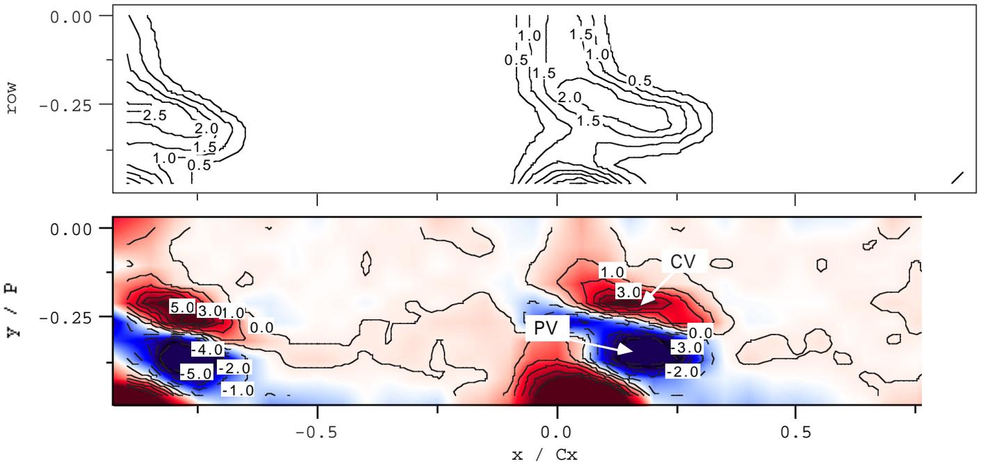
Fig. 8 Measurements of total loss and secondary vorticity distributions for the no-suction case at the slot #6
