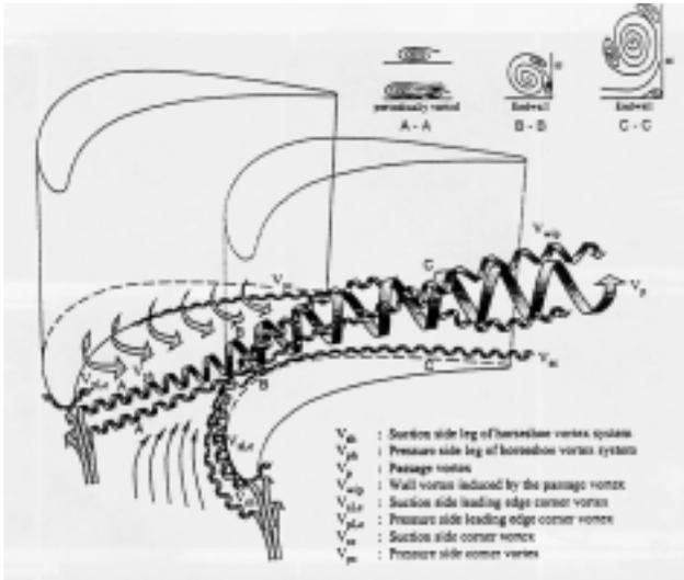
Fig. 1 Secondary flow model in a turbine cascade (Wang et al., 1995)
