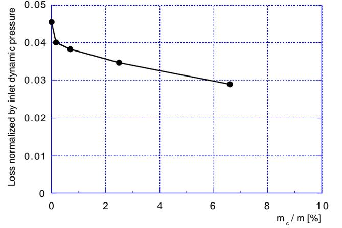
Fig. 12 Loss reduction by the endwall suction
