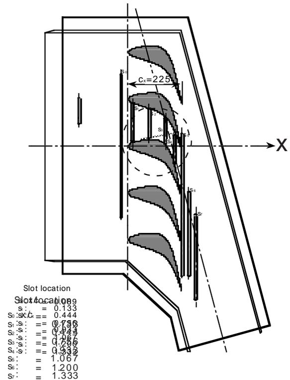
Fig. 3 Top view of the test cascade with the location of the measurement slots and suction slit
