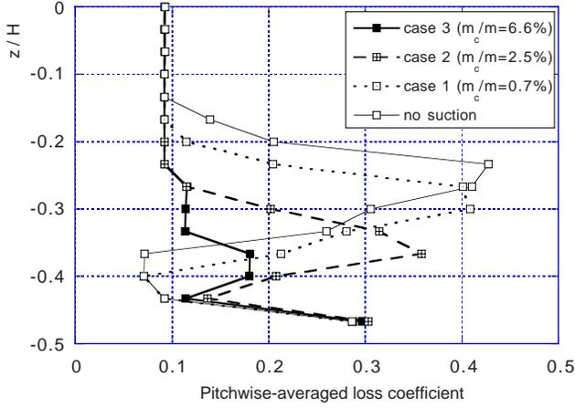
Fig. 11 Pitchwisely mass-averaged loss coefficient
