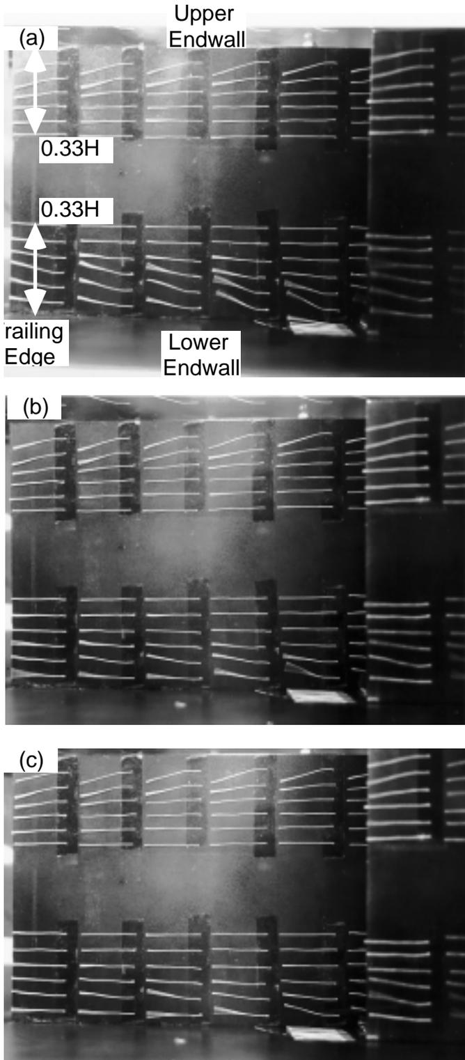
Fig. 5 Behaviors of tufts on the blade suction surface
