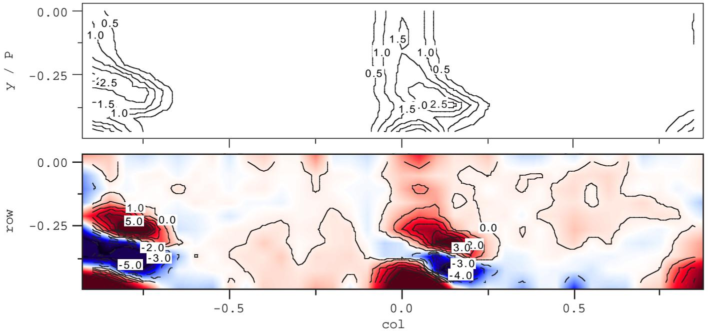
Fig. 9 Measurements of total loss and secondary vorticity distributions for medium suction case ( $P=0.933$ ) at the slot #6
