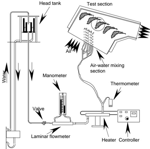
Fig. 4 Water supply system for simulation of water deposition on the outer casing of a steam turbine
