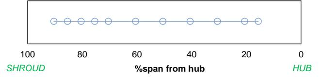
FIGURE 4. SPAN WISE MEASUREMENT LOCATIONS
