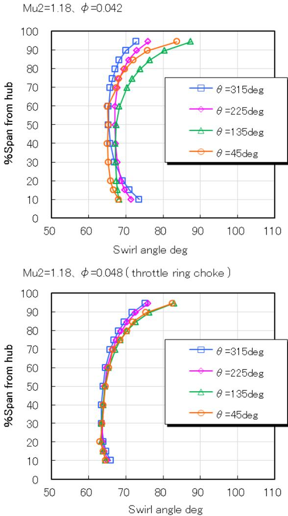
FIGURE 8. IMPELLER EXIT FLOW ANGLE CIRCUMFERENTIAL VARIATION ( $\theta =$  AZIMUTHAL ANGLE)
