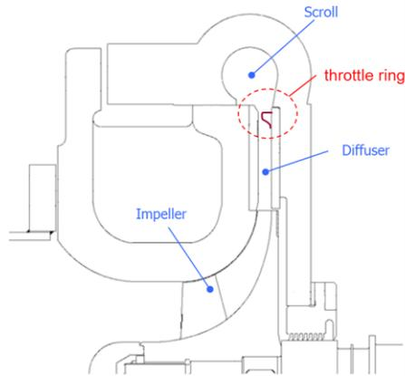
FIGURE 5. MERIDIONAL VIEW OF THE EXPERIMENTAL SETUP
