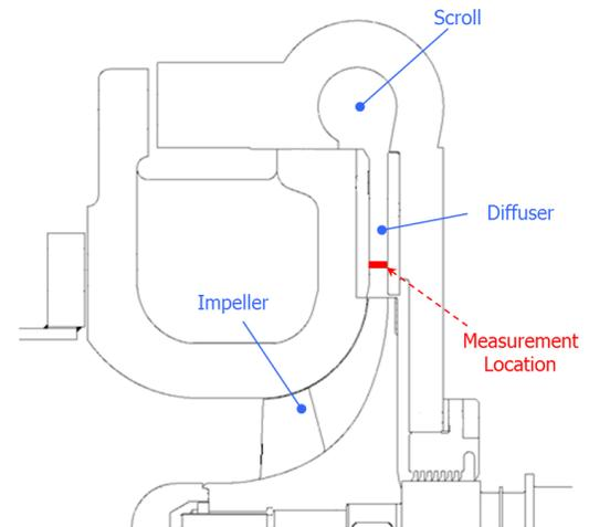
FIGURE 2. FLOW MEASUREMENT LOCATION 1.1 D2 CIRCUMFERENTIAL POSITION
