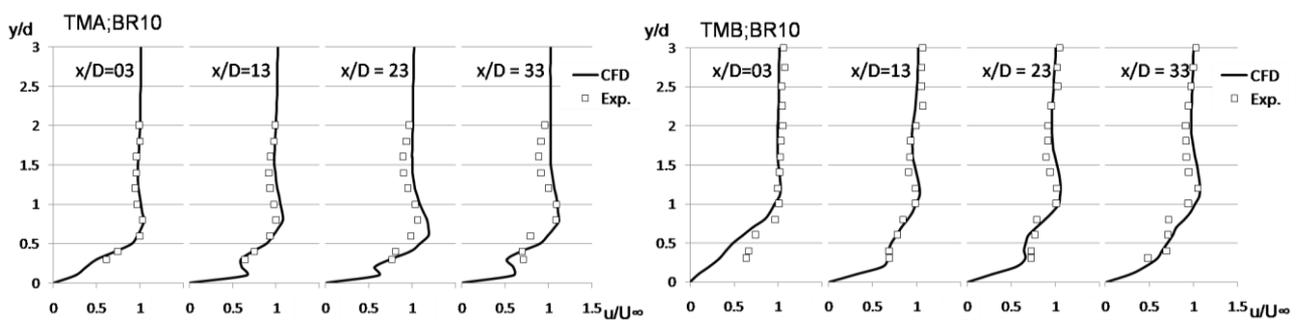
Fig. 6: Velocity profile comparison between the experiment and CFD
