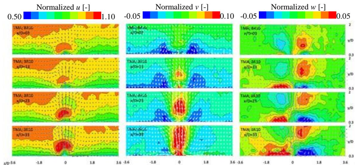
Fig. 5: Results of TMA; (a) Normalized  $u$  velocity, (b) Normalized  $v$  velocity, and (c) Normalized  $w$  velocity
