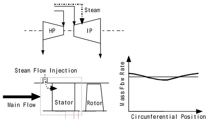
**Figure 1: Flow Injection Schematic Diagram.**
