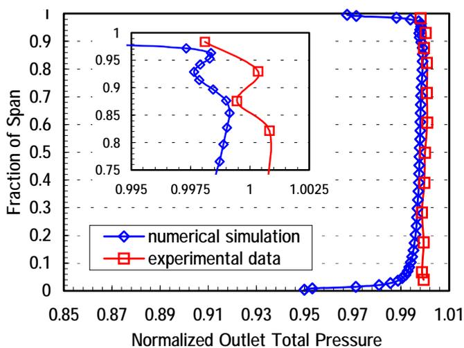
**Figure 4: Normalized outlet total pressure distribution.**
