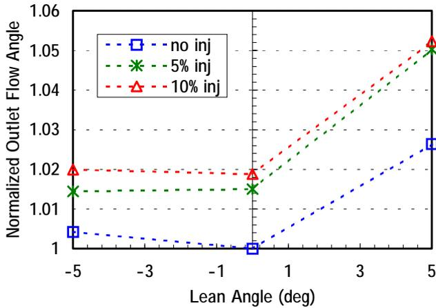
**Figure 8: Normalized outlet flow angle for the leaned nozzle vanes.**
