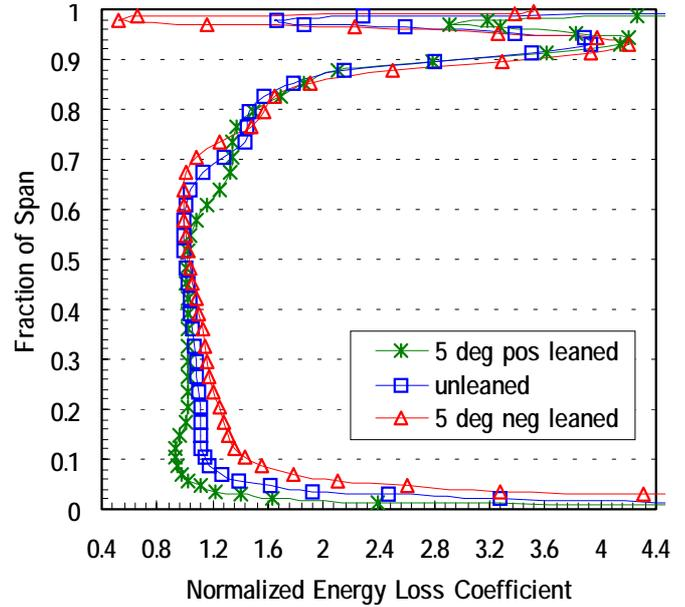
**Figure 9: Normalized pitchwisely mass-averaged energy loss coefficient for the 10% flow injection case.**
