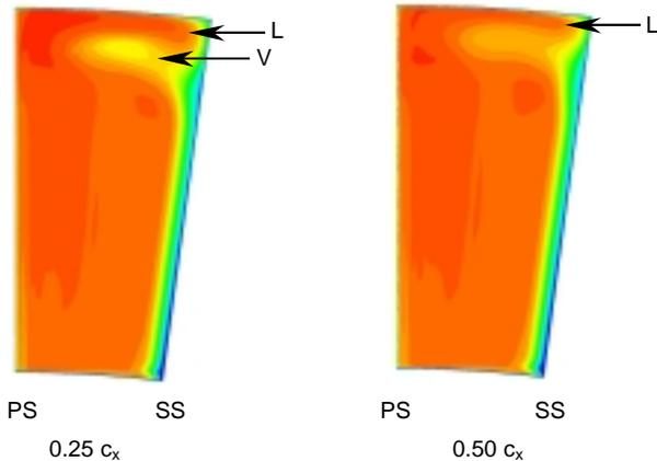
**Figure 17: Normalized total pressure distribution for the  $0.25c_x$  (left side) and  $0.5c_x$  (right side) cases with 10% flow injection for three streamwise locations.**
