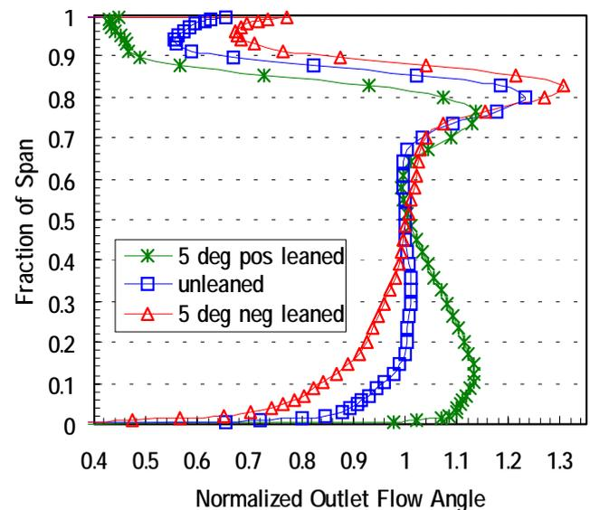
**Figure 7: Normalized pitchwisely mass-averaged outlet flow angle for the 10% flow injection case.**
