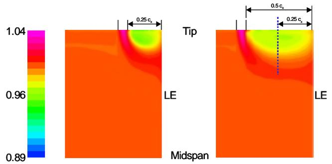
**Figure 16: Normalized total pressure distribution upstream the leading edge for the  $0.25c_x$  and  $0.5c_x$  cases (10% flow injection, 50% pitch).**
