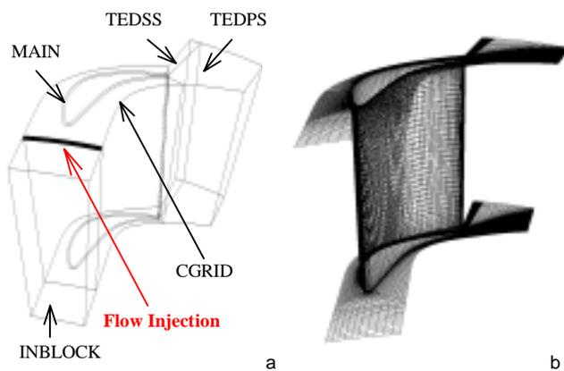
**Figure 3: Grid block configuration and grid system.**
