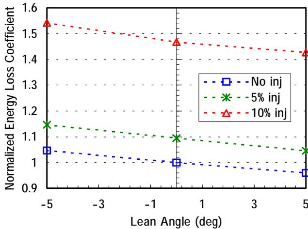
Figure 12: Normalized energy loss coefficient for the leaned nozzle vanes.
