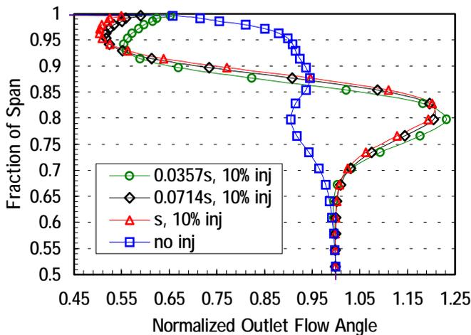
Figure 13: Normalized pitchwisely mass-averaged outlet flow angle for the 10% flow injection case.
