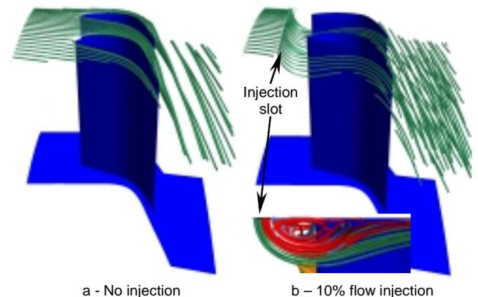
**Figure 5: Streaklines for the no injection and 10% flow injection cases.**
