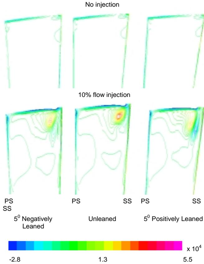
**Figure 11: Streamwise vorticity contours for no injection and 10% flow injection cases at 50% axial chord (from 70% span to tip).**
