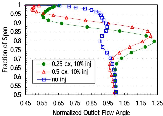
**Figure 15: Normalized pitchwisely mass-averaged outlet flow angle for the 10% flow injection case.**
