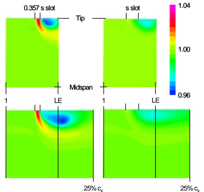
Figure 14: Total pressure distribution upstream the leading edge for the 10% flow injection case (top: 50% pitch, bottom: 0% pitch).
