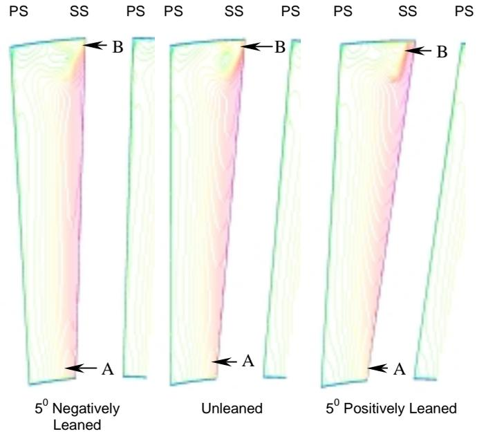
**Figure 10: Absolute velocity contours for the 10% flow injection case at 50% axial chord.**
