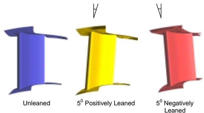
**Figure 2: Unleaned and leaned nozzle vanes.**
