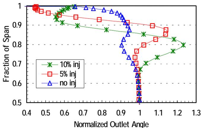
**Figure 6: Normalized pitchwisely mass-averaged outlet flow angle for the straight blade.**
