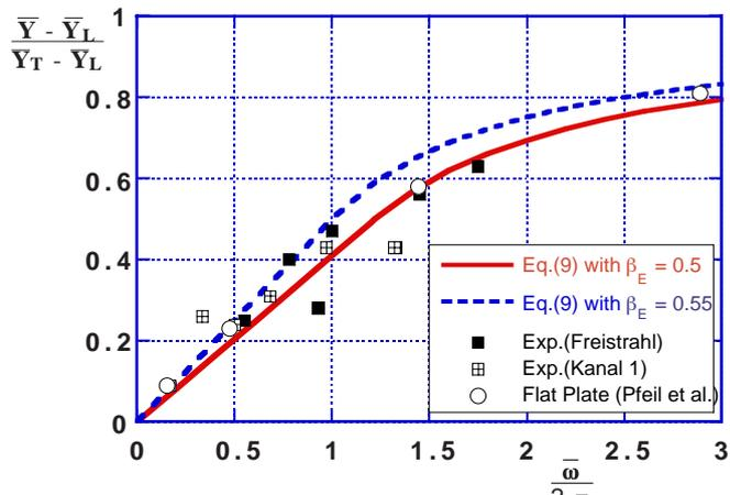
Figure 4 Comparison of the generalized Hodson's model and experimental data
