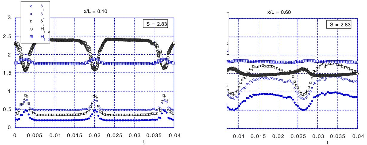
Figure 5 Time-resolved characteristics of the wake-affected boundary layer ( $S = 2.83$ ) (left)  $x/L = 0.10$  (right)  $x/L = 0.60$
