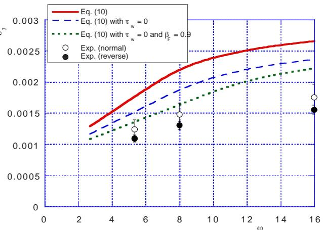
Figure 8 Wake-affected energy dissipation thickness at  $x/L = 0.6$  and the estimation
