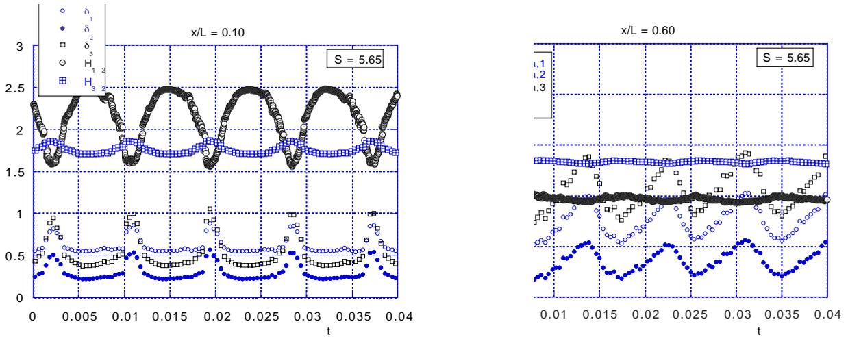
Figure 6 Time-resolved characteristics of the wake-affected boundary layer ( $S = 5.65$ ) (left)  $x/L = 0.10$  (right)  $x/L = 0.60$
