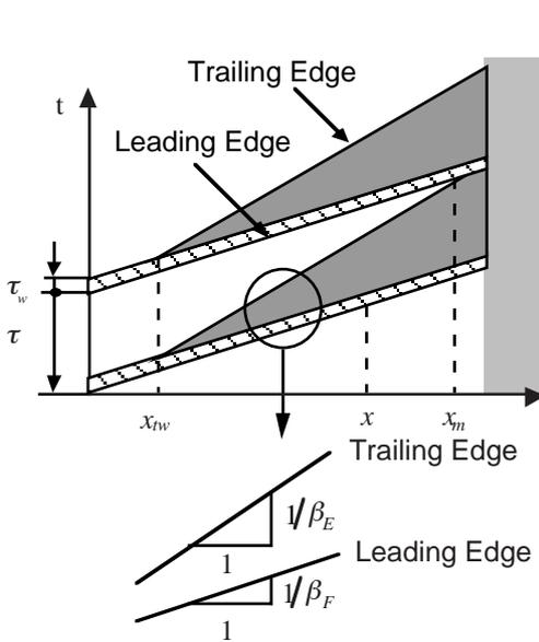
Figure 3 Distance-time diagram of the wake-affected boundary layer
