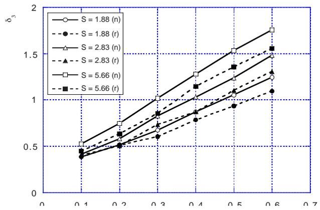
Figure 7 Time-averaged energy dissipation thickness for several unsteady conditions
