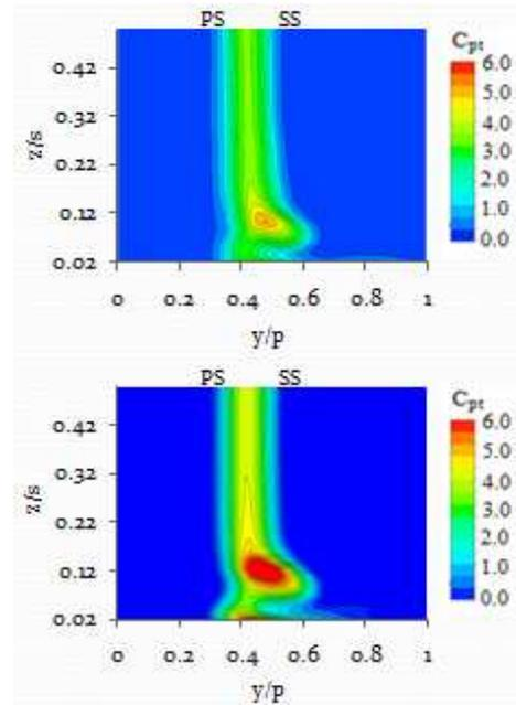
Fig. 4. Total pressure loss for baseline condition based on EFD(top) and CFD(bottom).
