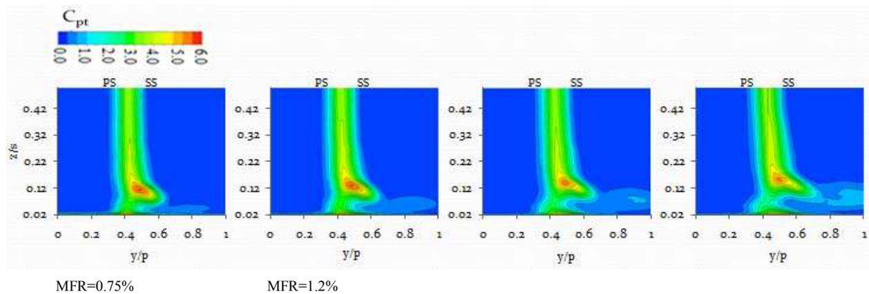
Fig. 5. Total pressure loss contours for each case based on EFD.
