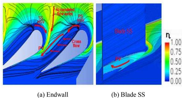
Fig. 9. Film cooling effectiveness on endwall (a) and blade SS (b) by CFD.
