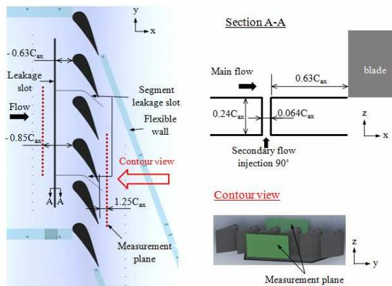
Fig. 1. Measurement area and slot geometry.
