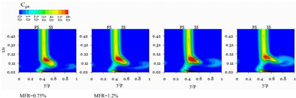
Fig. 6. Total pressure loss contours for each case based on CFD.
