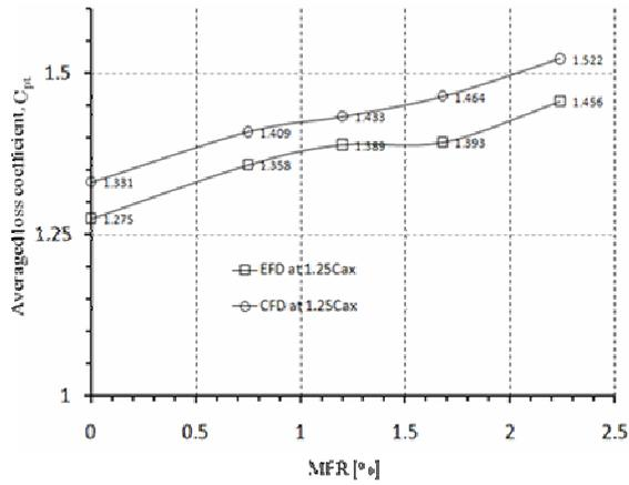
Fig. 7. Plane averaged total pressure loss,  $C_{pt}$ .
