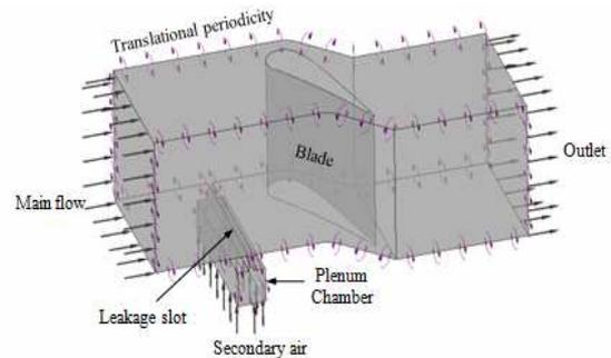
Fig. 2. Geometry of the CFD model.
