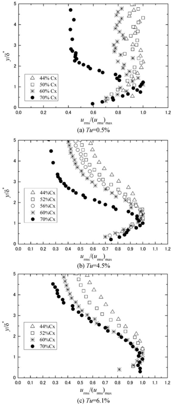
Fig. 5 RMS velocity fluctuation profiles ( $Re=170,000$ )
