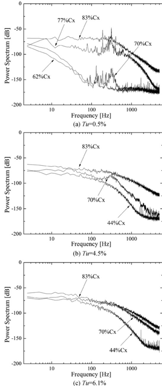
**Fig. 4** Power spectra of velocity fluctuation ( $Re=170,000$ )
