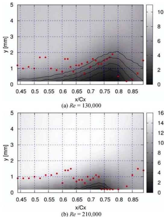
Fig. 7 Time-averaged velocity contours ( $Tu = 0.5\%$ )
