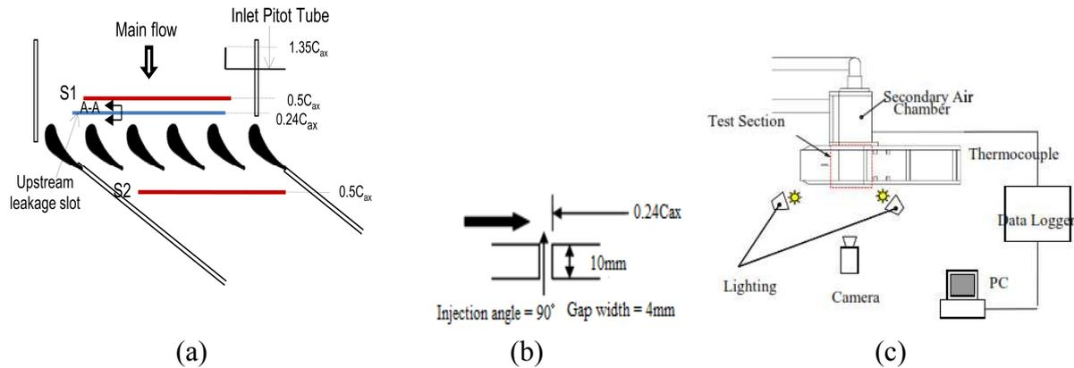
Fig. 1 Experimental setup for aerodynamic and heat transfer
