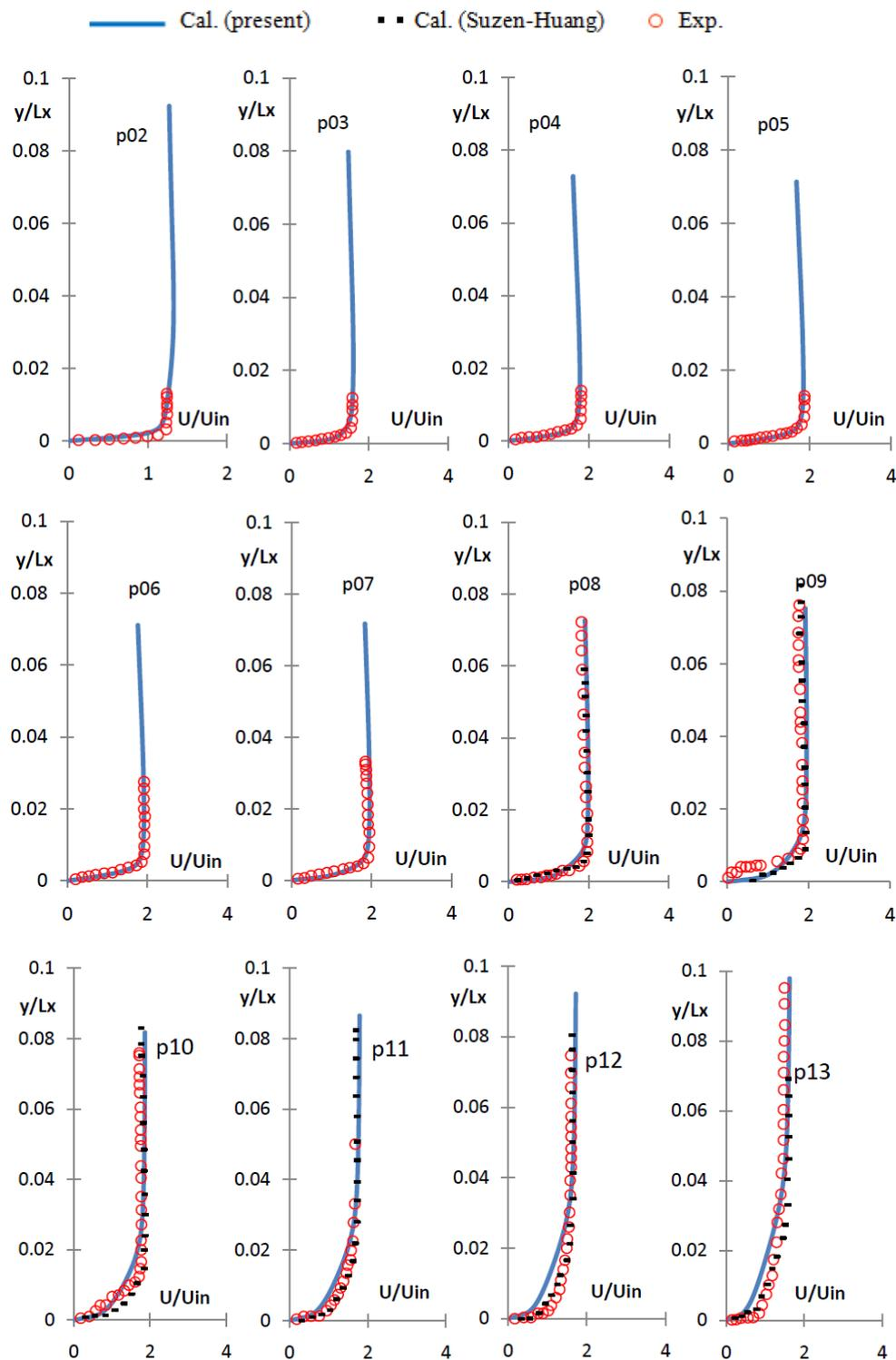
**Figure 7** Comparisons of velocity profile from p02-p13, for the case of  $Re = 3 \times 10^5$  and  $FSTI=2.5\%$
