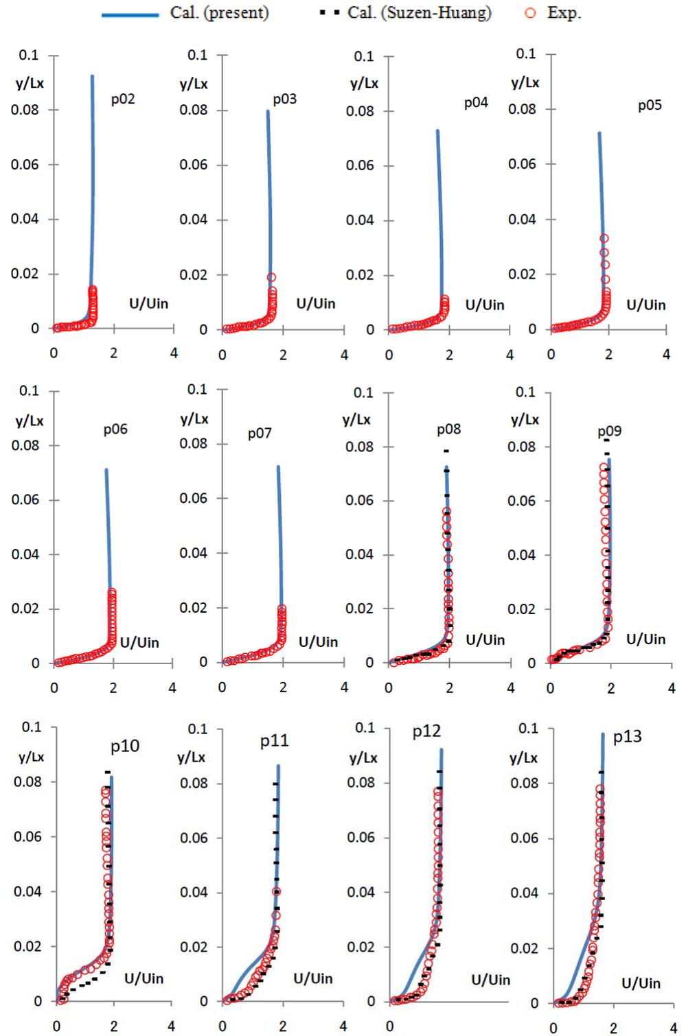
Figure 6 Comparisons of velocity profile from p02-p13, for the case of  $Re = 2 \times 10^5$  and  $FSTI=2.5\%$
