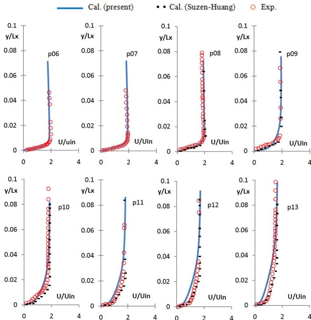
Figure 10 Comparison of velocity profile from p06-p13, for the case of  $Re = 2 \times 10^5$  and FSTI=10%
