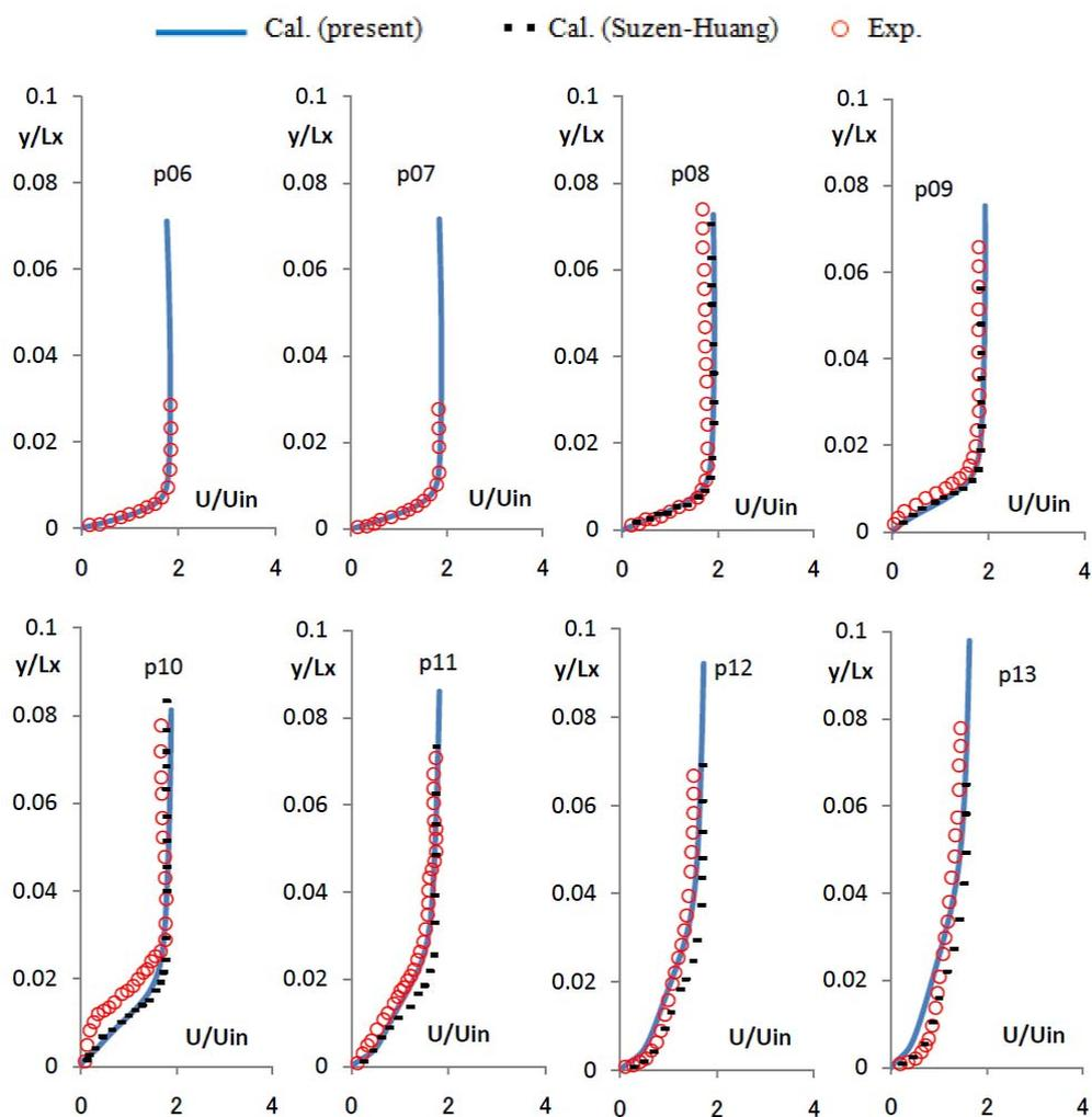
**Figure 9** Comparison of velocity profile from p06-p13, for the case of  $Re = 1 \times 10^5$  and  $FSTI=10\%$
