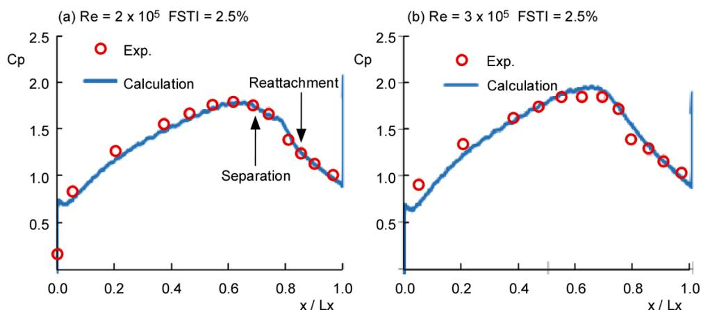
Figure 5 Comparisons of pressure coefficient for the cases of
