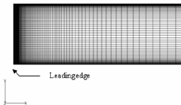
**Figure 1** Grid system used for flat plate simulations
