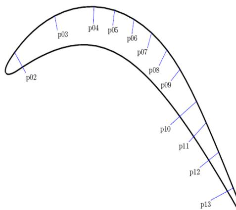
Figure 4 Pak-B airfoil geometry and measurement stations on the suction surface of the blade
