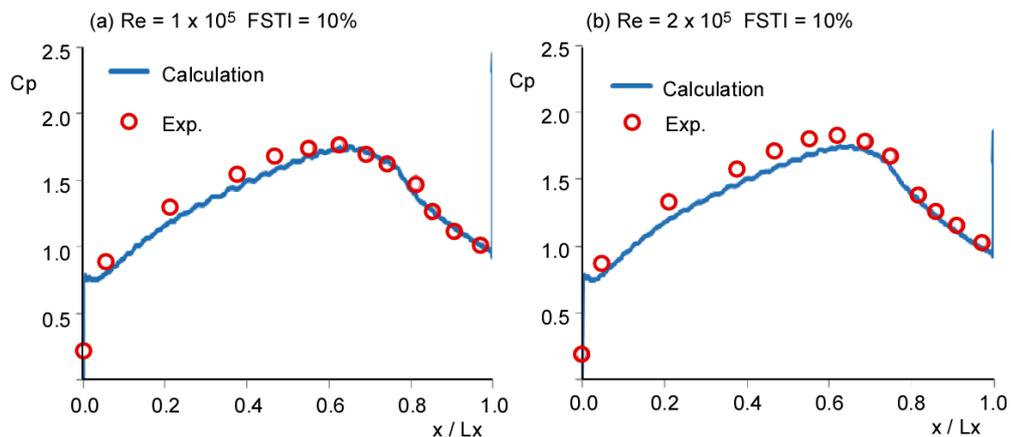
**Figure 8** Comparison of pressure coefficient for the case of (a)  $Re = 1 \times 10^5$  and  $FSTI=10\%$  (b)  $Re = 2 \times 10^5$  and  $FSTI=10\%$
